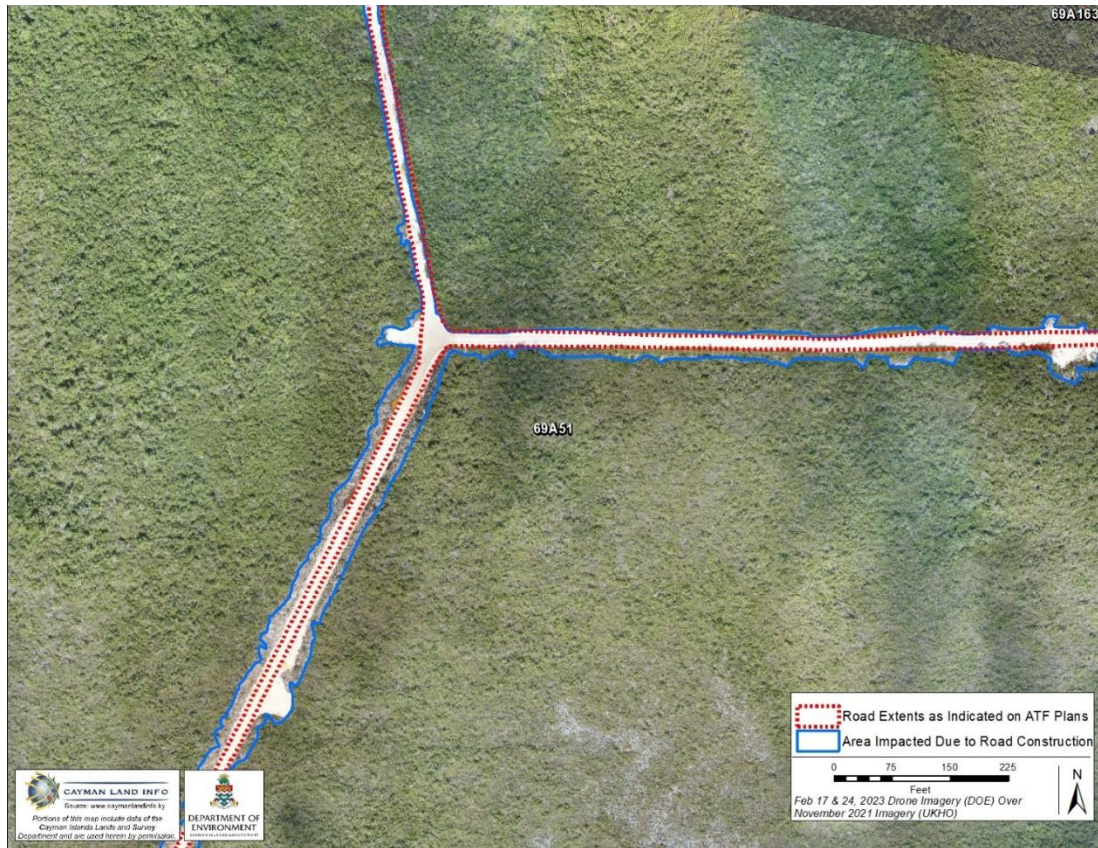
Figure 2. The survey drawing of the extent of the after-the-fact road is shown as red. However, the width of the road is wider than depicted (see the areas of white fill exposed on either side of the red dashed line) and the area impacted by clearing (blue) is even larger based on our drone imagery (Source: DoE, 2023).
