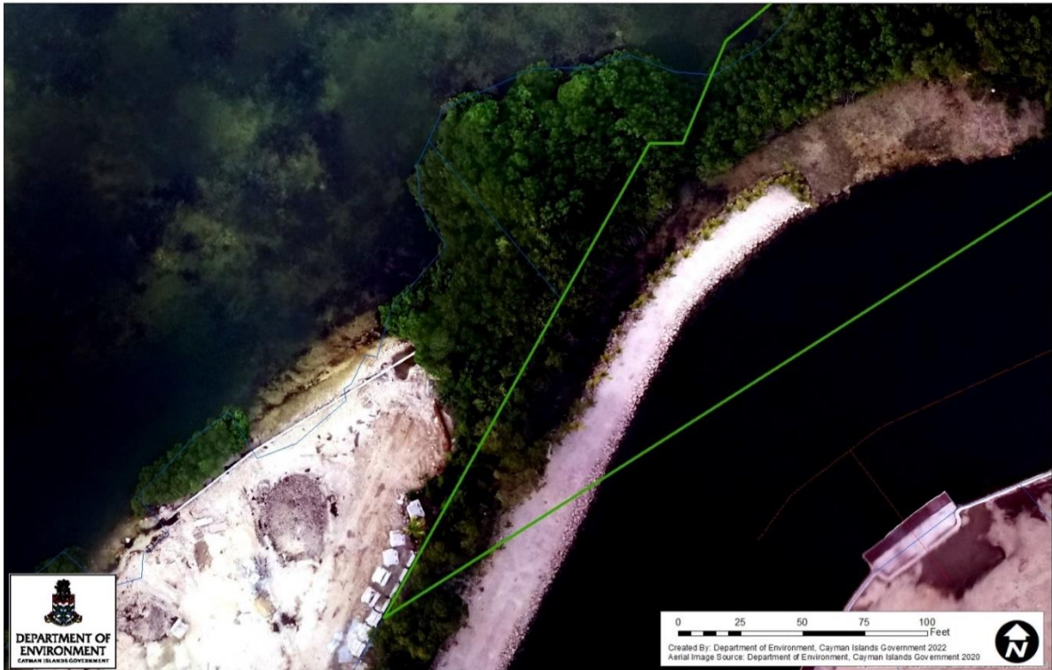
Figure 1: DOE Aerial Imagery showing the Mangrove Buffer Zone (outlined in green) and the filled road section and cleared area encroaching into it (DOE 2021).
